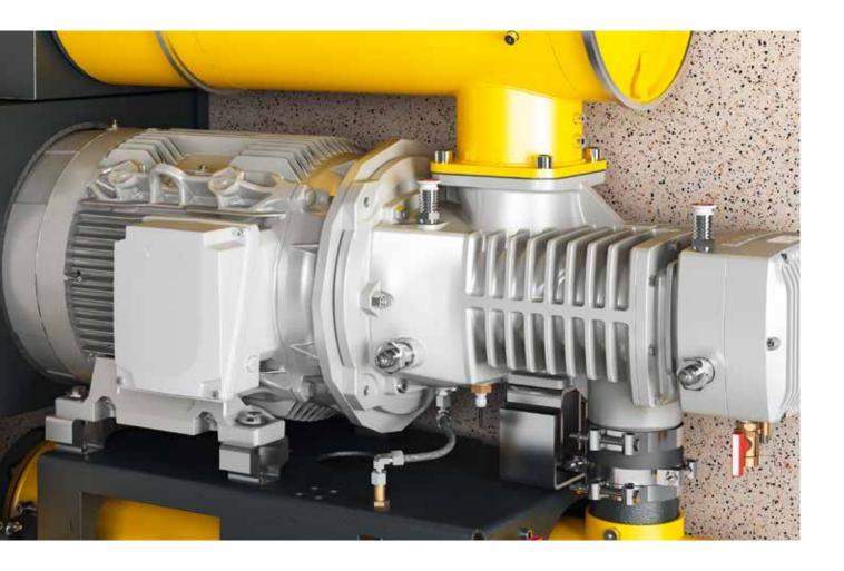
In CBS and DBS series rotary screw blowers, power is transferred from the motor to the blower airend via an integrated gear transmission. This was found to be the most effective transmission solution for the speeds in this power and size class with regards to efficiency, dependability and durability. With HBS series blowers, power is transferred directly without loss via a coupling. These concepts were the result of extensive research at KAESER's Research and Development Centres.
